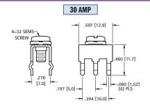
CAT. NO. 8197-SEMS (Screw Supplied Unassembled) CAT. NO. 8199-SEMS (Screw Installed & Captivated)
