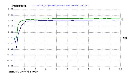
Wetting balance test results for Nicolloy<sup>™</sup> tested as received using an ROL1 flux from a popular solder paste.
