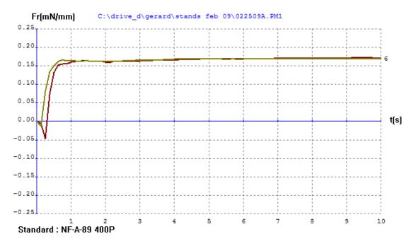
Wetting balance test results for Nicolloy<sup>™</sup> tested as received using an ROL1 flux from a popular solder paste – The improvement in wetting is dramatic with good wetting forces, quick wetting times and post test visual examination of the devices showing excellent uniform coating of the terminals by the solder.
