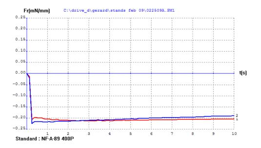
Wetting balance test results for Nicolloy<sup>™</sup> tested as received using the Standard 0.2% test flux (ROL1) per the ANSI J-STD-002 - the part does not produce sufficient forces to cross the buoyancy line and produce positive wetting. Visual inspection of the parts post testing show non wetting to the surface of the terminals in the majority
